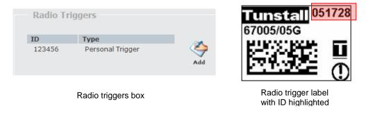
**Note:** This feature is only available for 869MHz telecare radio receivers on the RS485 bus. For more information on how your scheme has been installed please contact your manager. If a radio trigger has already been added to a resident via the SCP then the details of the trigger will appear in the web browser these details can then be altered if required.
