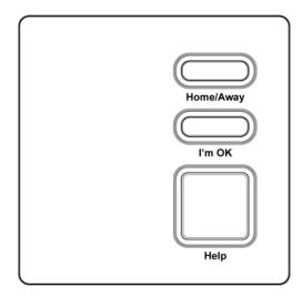
In addition to the red alarm button, speech modules with 3 buttons have a Home/Away button which is used to turn the away mode on and off. An away light is also provided to clearly indicate to the user which state the module is in. The I'm OK button can be used to signal to the scheme manager/ control centre that the resident is active (It does not raise a call).
