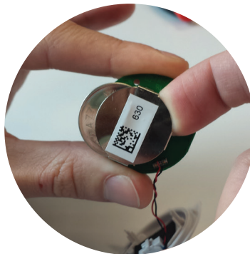
5) Slide the battery out of the battery holder by pushing it from the side using your finger. Do not use a conductive object such as a metal screw driver.
