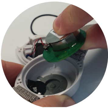
4) Lift the PCB by holding the battery holder
