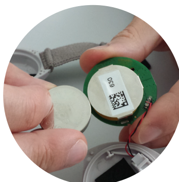
6) Slide in the new CR2477 battery into the holder, with the "+" face up
